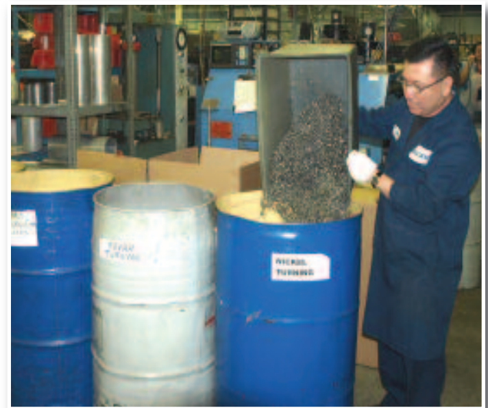
Nickel alloy chips are poured into the appropriate barrel for recycling in the NC machining department.
