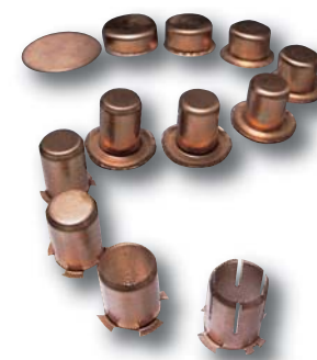
Twelve stations bring this part from blank to completion.
