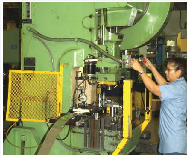
This coil-fed press is set up for a long production run.
