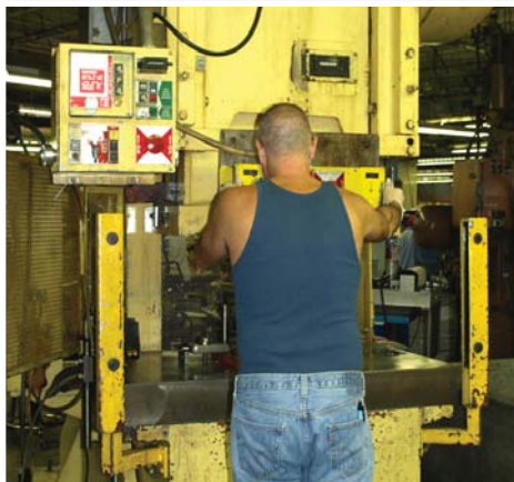
A stamping press is prepared for a progressive die at Gasser.
